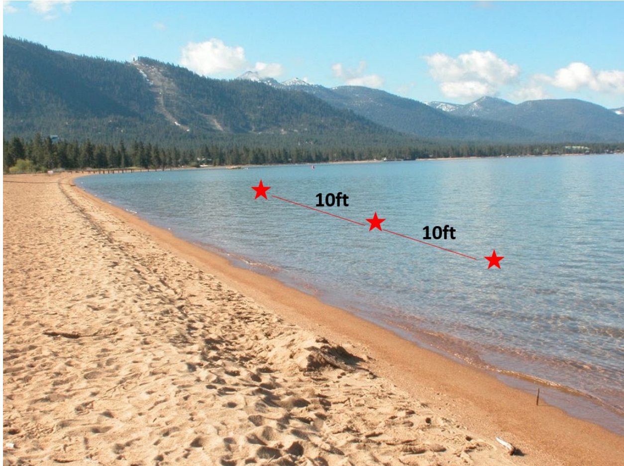
Figure 1. Transect sampling method for lakes. Collect three samples at knee depth 10 feet apart, walking parallel to shore.
